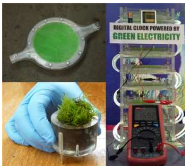
Figure 2. Current BPV prototypes produced at the University of Cambridge. Algae (top left and right) and moss (bottom left) designs can presently produce enough energy to power small electronic devices.
